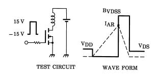
$$\begin{aligned} R_G &= 25~\Omega \\ V_{DD} &= 90~V,~L = 7.98~mH \end{aligned} \qquad E_{AS} &= \frac{1}{2} \cdot L \cdot I^2 \cdot \left( \frac{B_{VDSS}}{B_{VDSS} - V_{DD}} \right) \end{aligned}$$
